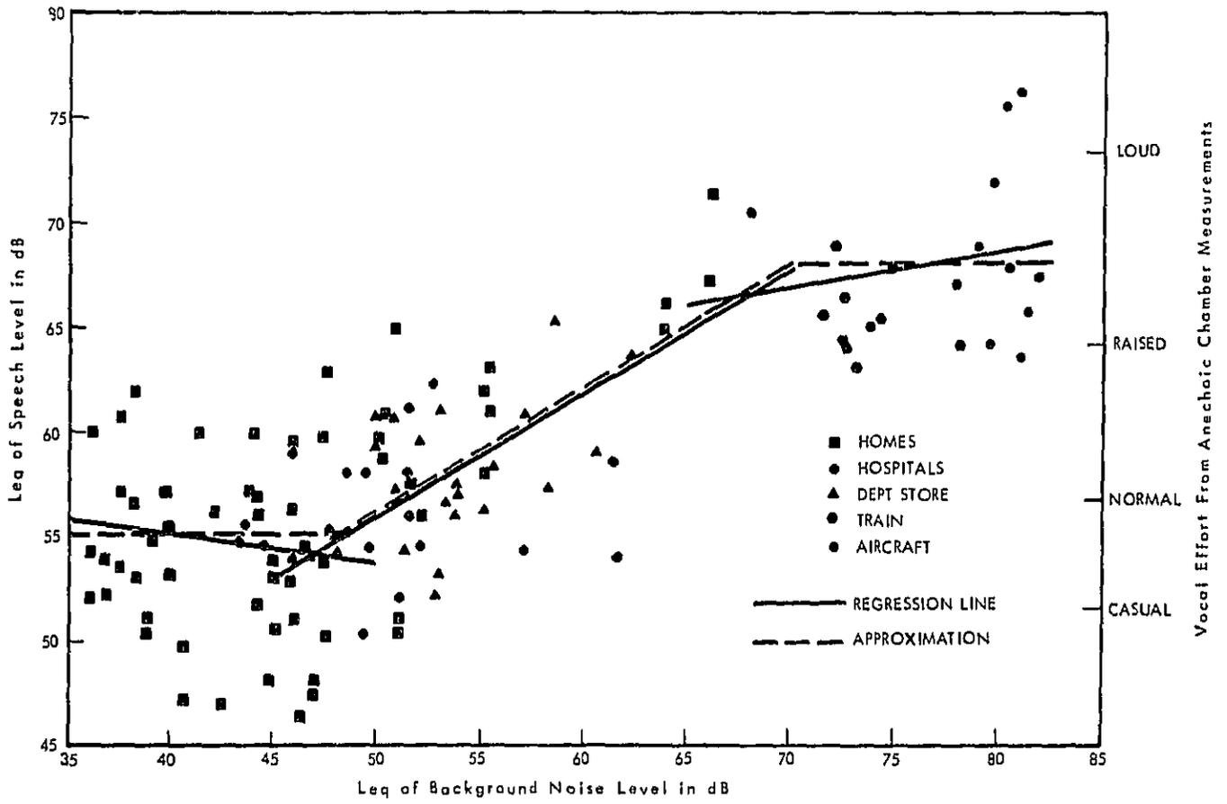
FIGURE 21. CONVERSING SPEECH LEVEL NORMALIZED TO ONE METER AS A FUNCTION OF BACKGROUND NOISE IN SEVERAL ENVIRONMENTS
