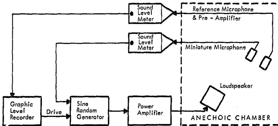
A-3 EQUIPMENT SETUP FOR CALIBRATION OF MINIATURE MICROPHONE USED IN CONVERSATIONAL SPEECH RECORDING
