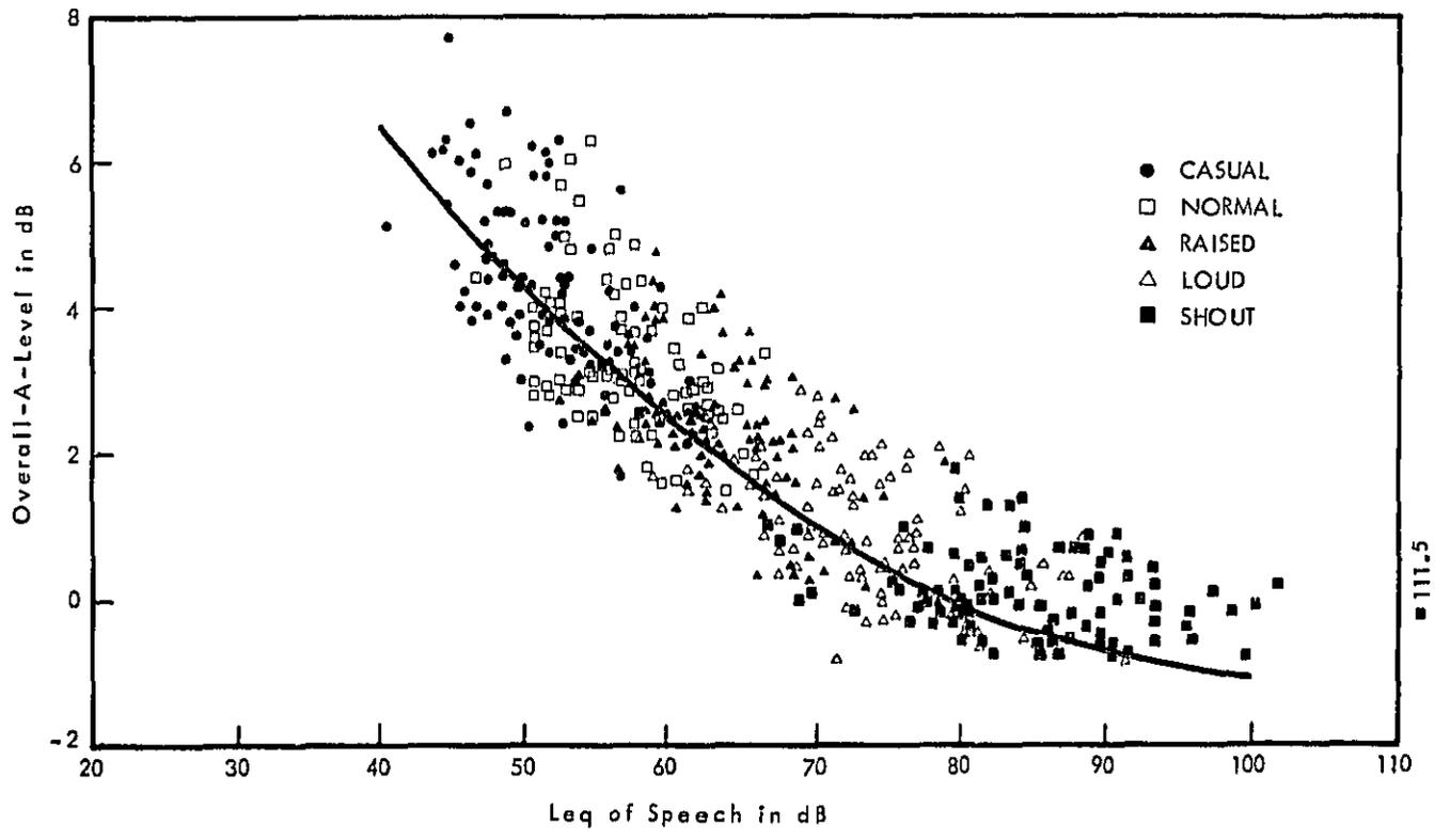
FIGURE 19. DIFFERENCES BETWEEN OVERALL AND A-WEIGHTED SOUND PRESSURE LEVELS OF SPEECH
