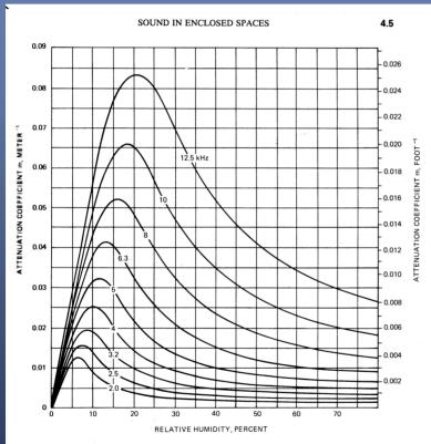
FIG. 4.2 Values of the total attenuation coefficient m vs. percent relative humidity for air at arc and normal atmospheric pressure for frequencies between 2000 and 12,500 Hz. Values of m regiven in both SI units and U.S. Customary System units. (After C. M. Harris. 1.2)
