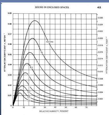
FIG. 4.2 Values of the total attenuation coefficient m vs. percent relative humidity for air at DFC and normal atmospheric pressure for frequencies between 2000 and 12,500 Hz. Values of m me given in both SI units and U.S. Customary System units. (After C. M. Harris. <sup>(2)</sup>)
