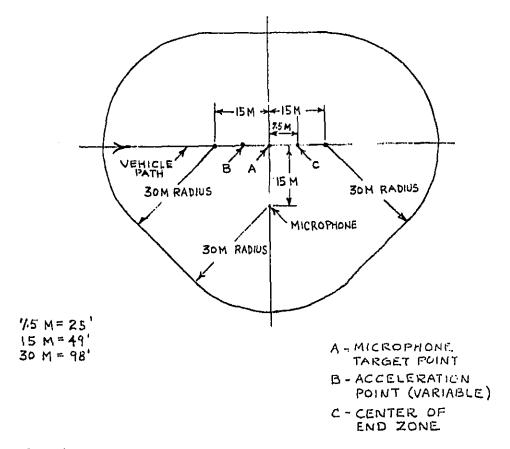
FIG. 1 - TEST MEASUREMENT AREA , PROCEDURE NO. F-76a
