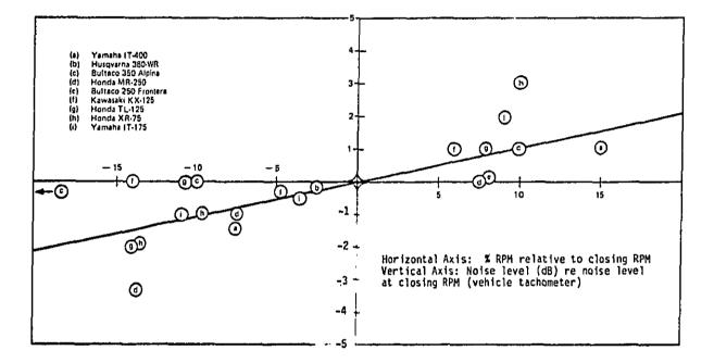
FIGURE I-3 NOISE LEVEL AS A FUNCTION OF CLOSING RPM OFF-ROAD MOTORCYCLES (including trials and mini-cycles)
