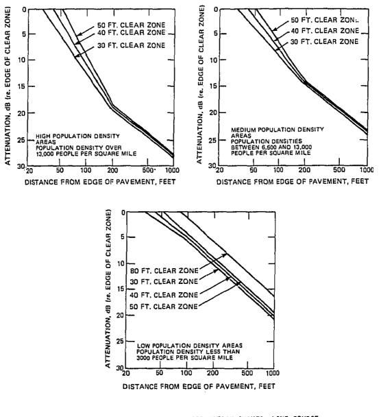
FIGURE N-2 SOUND LEVEL ATTENUATION CURVES: LINE SOURCE
