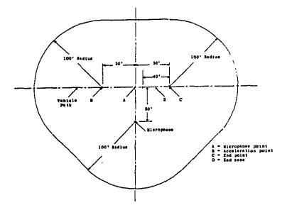
Fig. 3-3. Test Area Layout for Heavy Trucks and Buses
