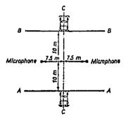
Fig. 1. — Monowing positions for measurement with vehicles in motion
