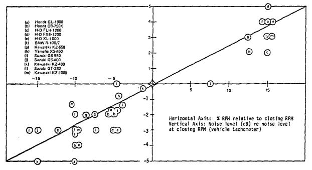
FIGURE I-1 NOISE LEVEL AS A FUNCTION OF CLOSING RPM STREET MOTORCYCLES
